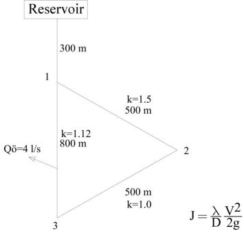
**QUESTION 4:** Design the main and primary pipes of the network by using Dead End Method for the water network supplying the water demand of a town with a population of 2ba00 given in the figure below. Use Hazen-Williams equation ( $V = 0.85CR^{0.63}J^{0.54}$ ) with a coefficient of C=130 (for cast iron pipes). (Standard Pipe Diameters are; 80m, 100mm, 125mm, 175mm, 200mm, 250mm, 300mm, ....).
