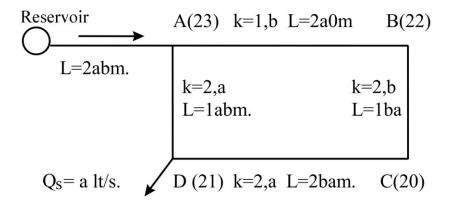
**QUESTION 2:** The following water network supplies the water demand of a town with a population of 2ab00. Estimate the main and primary pipe diameters by using Dead End method. Use Colebrook-White Tables in the calculations. Pipe lengths and population density coefficients are given on the figure. (meanq<sub>day</sub>= 1ba l/day/capita, Minimum allowable pressure (P/ $\gamma$ )<sub>min</sub>=30 mwc, Maximum allowable pressure (P/ $\gamma$ )<sub>max</sub>=80 mwc).
