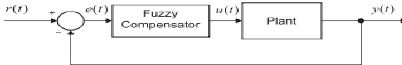
Figure 4.1. Closed-loop system with cascade fuzzy controller.
