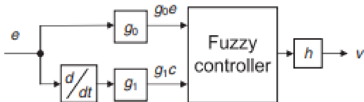
Figure 4.10. Fuzzy compensator block of Figure 4.9.
