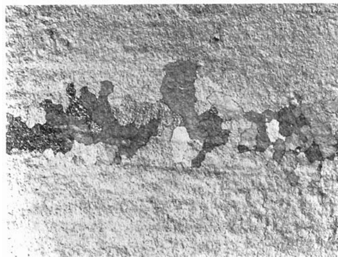
Fig. 7.10 A freckle line on the surface of a nickel-base superalloy casting (Giamei and Kear 46 ).
