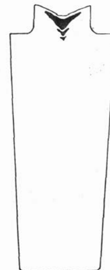
Fig. 9.23 Cross section of a killed steel ingot cast into a mould with a refractory hot top (schematic). Shrinkage is confined to the top of the ingot and yield is increased.
