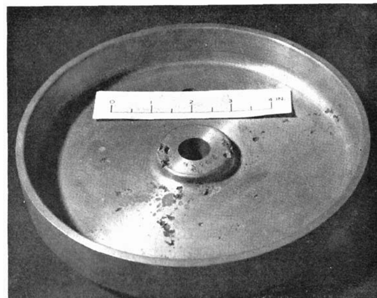
Fig. 9.7 Blowholes produced by reaction between the molten metal and entrapped slag. These generally have discoloured surfaces and are associated with slag
