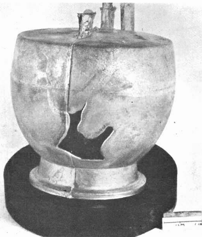
Fig. 9.24 A misrun in a brass gravity die casting.
