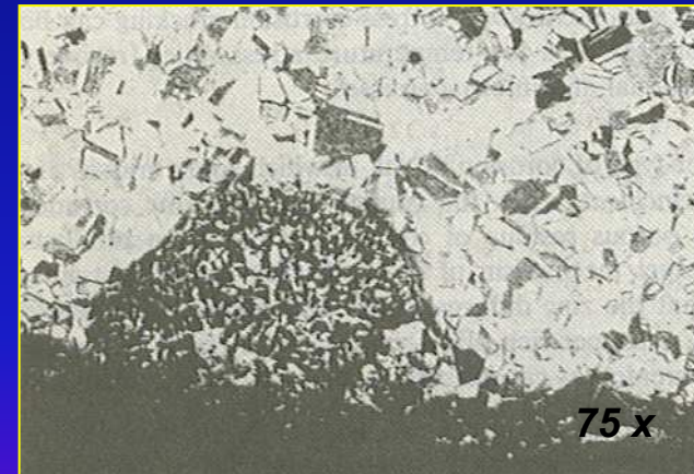
Dezincification of cartridge brass (70%Cu-30%Zn)
