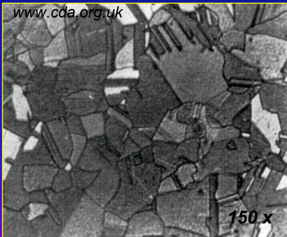
Microstructure of hot rolled deoxidised copper
