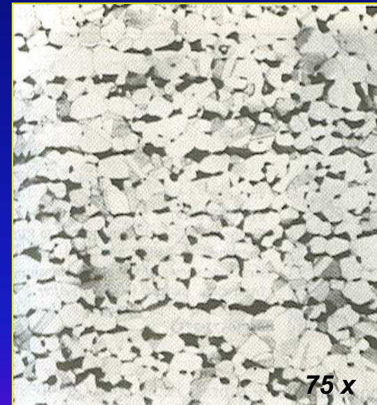
(b) Hot rolled Muntz metal sheet structure of beta phase (dark) and alpha phase (light)
