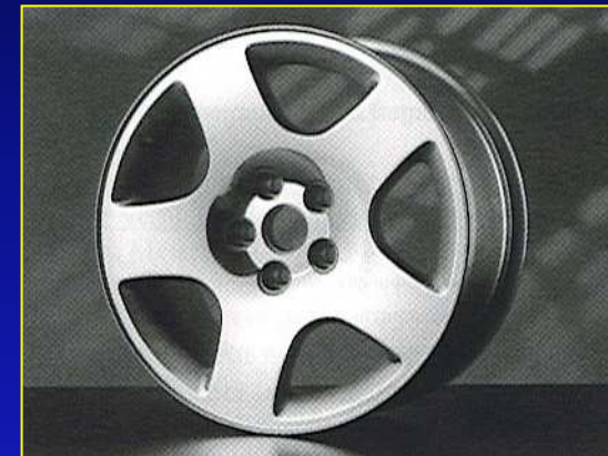
Prototype of a magnesium forged wheel(ZK30)
