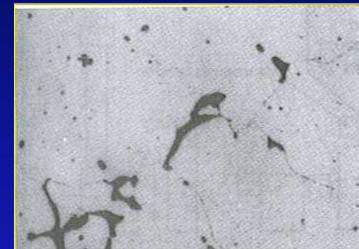
Binary Mg-Zn alloy treated at 330°C/8h
