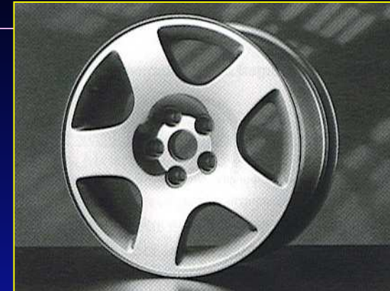
Prototype of a magnesium forged wheel(ZK30)
