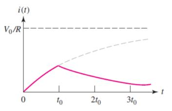
the time constant is only one half as large as the length of the applied pulse; the rising portion of the exponential has therefore almost reached V<sub>0</sub>/R before the decaying exponential begins. ( $\tau = t_0/2$ )
