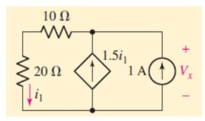
Circuit for finding the Thévenin equivalent of the network connected to the capacitor
