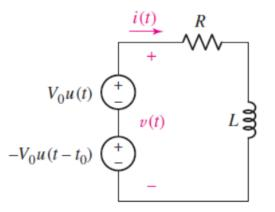
A rectangular voltage pulse which is to be used as the forcing function in a simple series *RL* circuit.
