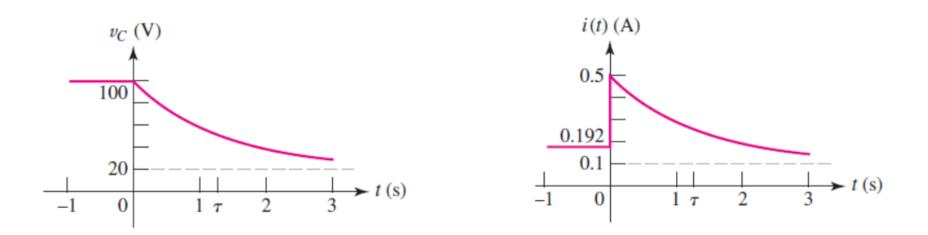
four numbers are needed to write the functional form of the response for this single energy-storage-element circuit, or to prepare the sketch: the constant value prior to switching (0.1923 ampere), the instantaneous value just after switching (0.5 ampere), the constant forced response (0.1 ampere), and the time constant (1.2 s). The appropriate negative exponential function is then easily written or drawn.
