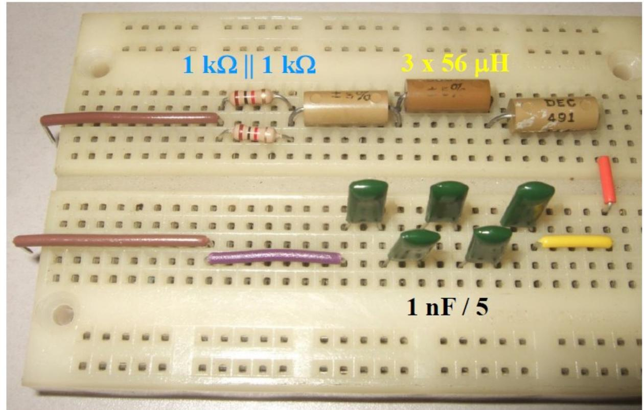
For a circuit that contains at least one sinusoidal source...
