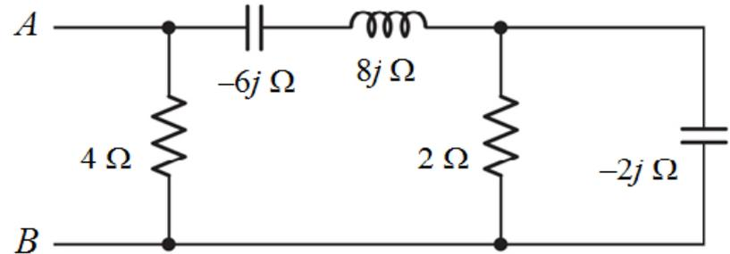
$$\begin{aligned} \mathbf{Z}_{A-B} &= \frac{\mathbf{Z}_2(4)}{(\mathbf{Z}_2 + 4)} = \frac{(1+j)(4)}{1+j+4} \\ &= \frac{4+4j}{5+j} = \frac{\sqrt{32} \angle 45.0^\circ}{\sqrt{26} \angle 11.3^\circ} = \end{aligned}$$
