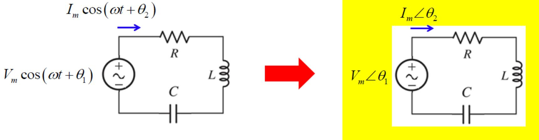
$$V_m \cos(\omega t + \theta_1) = \text{Re}\{V_m e^{j(\omega t + \theta_1)}\} = \text{Re}\{V_m e^{j\omega t} e^{j\theta_1}\} \Rightarrow V_m e^{j\theta_1} = V_m \angle \theta_1$$
