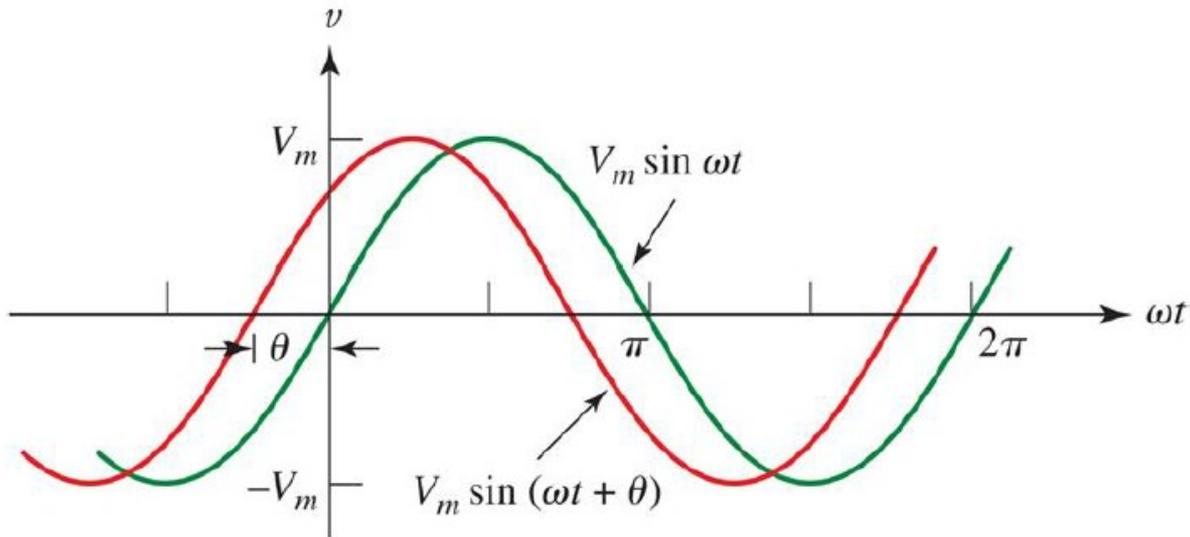
$v_2$  “leads”  $v_1$  by  $\theta$
