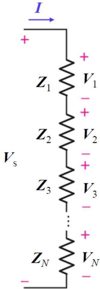
$$\begin{aligned}V_s &= V_1 + V_2 + V_3 + \dots + V_N \\ &= \mathbf{I}[\mathbf{Z}_1 + \mathbf{Z}_2 + \dots + \mathbf{Z}_N] \\ &= \mathbf{I} \cdot \sum_{n=1}^N \mathbf{Z}_n\end{aligned}$$
