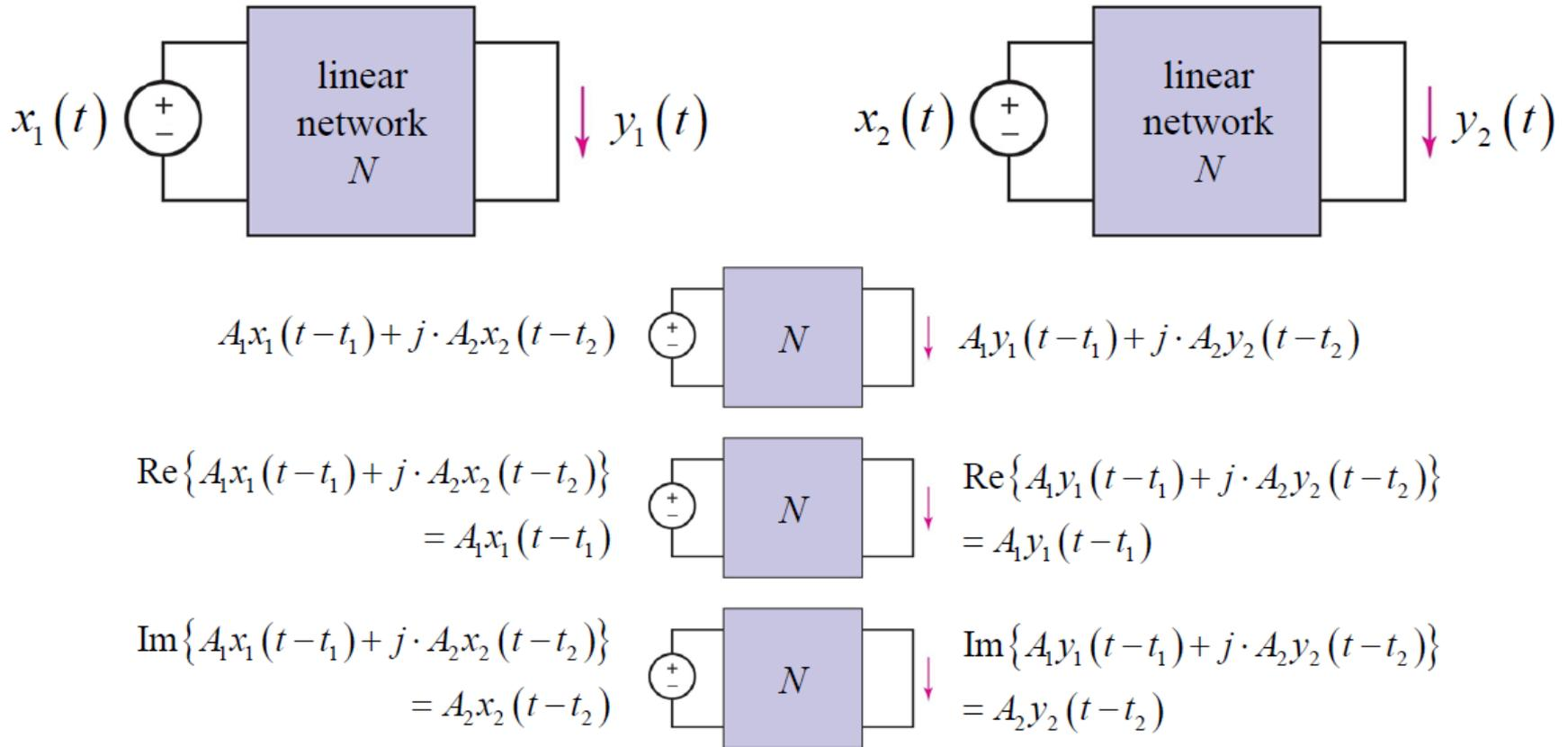
The real part of the response is caused by the real part of the source(s).
