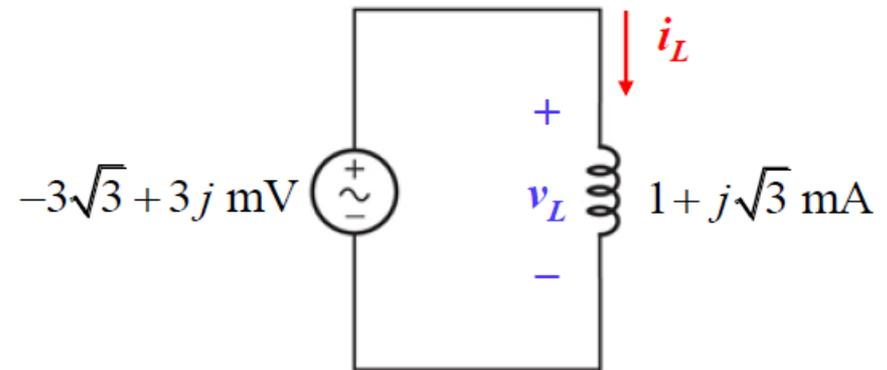
$$\begin{aligned} \frac{v_L}{i_L} &= \frac{-3\sqrt{3} + 3j \text{ mV}}{1 + j\sqrt{3} \text{ mA}} \\ &= \frac{\sqrt{(3\sqrt{3})^2 + (3)^2} \angle \tan^{-1}\{1/-\sqrt{3}\}}{\sqrt{(1)^2 + (\sqrt{3})^2} \angle \tan^{-1}\{\sqrt{3}\}} = \frac{6 \angle 150^\circ}{2 \angle 60^\circ} \end{aligned}$$
