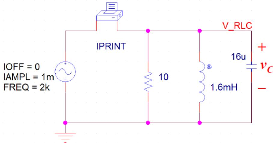
$$v_c(t) = e^{-\alpha t} [V_1 \cos(\omega_d t) + V_2 \sin(\omega_d t)] + V_3$$
