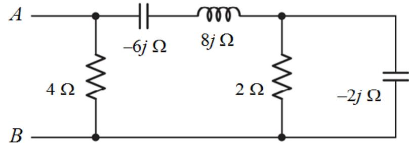
$$\mathbf{Z}_1 = \frac{(2)(-2j)}{(2-2j)} = \frac{4\angle -90^\circ}{\sqrt{8}\angle -45^\circ} = \sqrt{2}\angle -45^\circ = 1 - j\ \Omega$$
