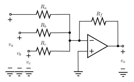
In the figure above,  $R_a$ =1k $\Omega$ ,  $R_b$ =2k $\Omega$ ,  $R_c$ =3k $\Omega$ .  $R_f$ =12k $\Omega$ . The sources are  $v_a$ =-4V,  $v_b$ =+2V, and  $v_c$ =1V. The power supplies for the op-amp are +15V and -15V. What is the value of  $v_o$ ? Notice that this op amp circuit might saturate, and you need to consider that possibility in your answer.
