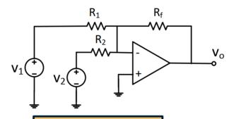
$$V_{0} = G_{1}V_{1} + G_{2}V_{2}$$
