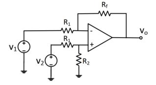
$$V_0 = \frac{R_F}{R_1} (V_2 - V_1)$$
