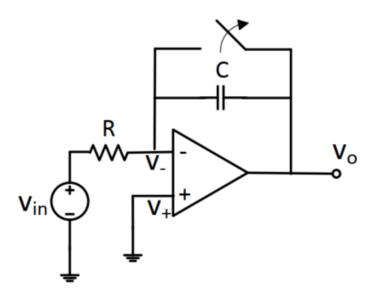
$$V_{o} = \frac{-1}{RC} \int_{0}^{t} V_{in} dt$$
