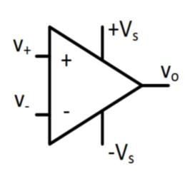
$$v_0 = A(v_+ - v_-)$$
