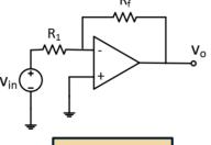
$$V_{o} = -\frac{R_{f}}{R_{1}}V_{in}$$
