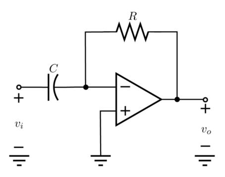
For the circuit above, R=5k $\Omega$  and C=2 $\mu$ F. If  $v_i$ =sin(1000t)V, what is the value of  $v_o$  at t=4 $\pi$ /3 ms?
