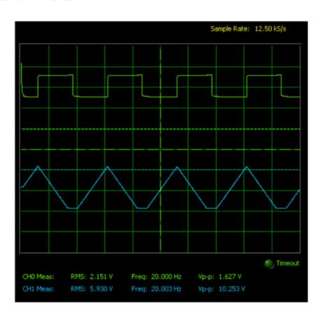
$$V_o = \frac{-1}{RC} \int_0^t V_{in} dt$$
