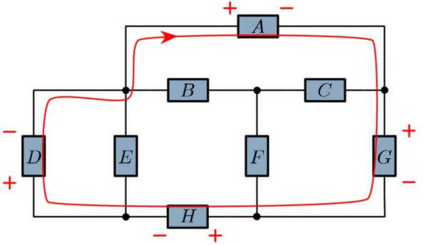
The sum of voltages around any closed loop is zero.
