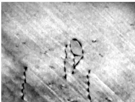
Dislocation generation through cross slip mechanism during in situ TEM deformation of alpha-titanium
