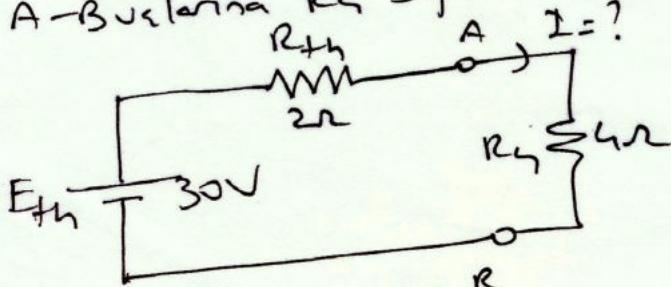
$$\frac{1}{R_{th}} = \frac{1}{6} + \frac{1}{12} + \frac{1}{4} = \frac{6}{12} \Rightarrow R_{th} = 2\Omega$$
