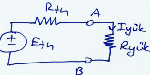
$$R_{yük} = R_{th} \Rightarrow I_{yük} = \frac{E_{th}}{R_{th} + R_{yük}} = \frac{E_{th}}{2R_{th}}$$
