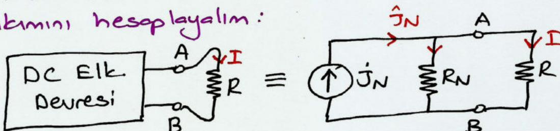
$$I = \frac{V_{AB}}{R} \quad \text{ve} \quad V_{AB} = R_{\text{es}} \cdot j_N = \left( \frac{R_N \cdot R}{R_N + R} \right) \cdot j_N$$
