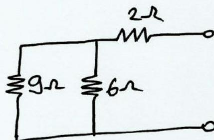
$$R_N = R_{ab} = 2 + \left( \frac{6 \cdot 9}{6+9} \right) \Rightarrow R_N = 5,6\Omega$$
