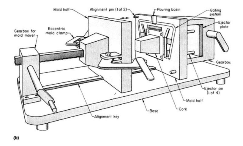
Two types of manually operated permanent mould casting machines. (a) Simple book-type mould for shallow-cavity castings. (b) Device with straight-line retraction for deep-cavity moulds.
