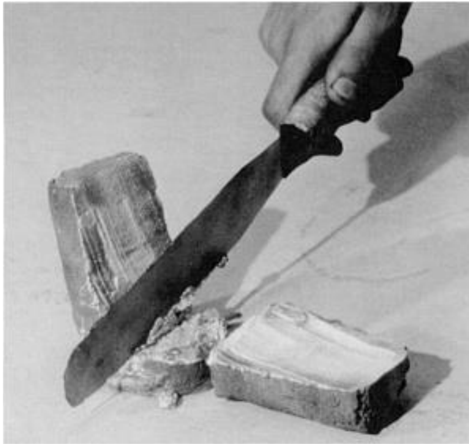
Semi solid aluminium billet being cut by a spatula
