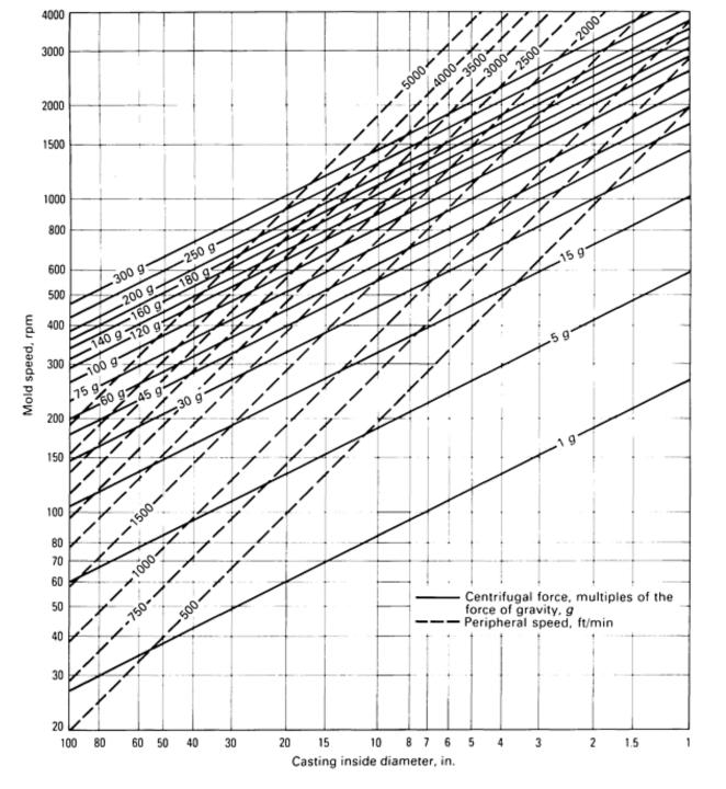
Nomograph for determining mould speed based on the inside diameter of the casting and the required centrifugal force. See text for example of use. **Mould Speed Curves.** Mould speeds are determined by the inside diameter of the castings to be made. The mould speed curve shown in nomograph is based on the inside diameter of the casting. The length of the casting is not considered in determining mould speed.
