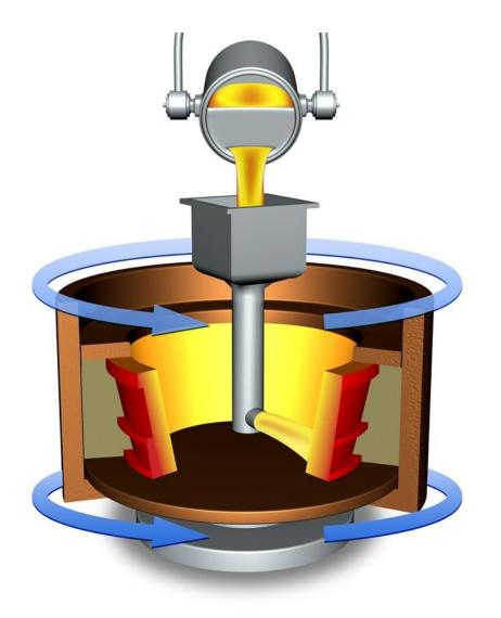
Vertical centrifugal casting machines are used for producing bushings and castings that are relatively large in diameter and short in length. The usual maximum length of the casting is two times the outside diameter of the casting. Vertical axis machines are also used for producing castings of odd or asymmetrical configurations.
