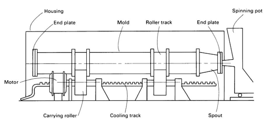
Schematic of a common design for a horizontal centrifugal casting machine
