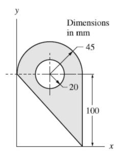
Fort he area in Fig, calculate the radii of gyration about the x- and y-axes
