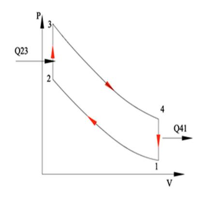
Below listed data are provided for a four stroke internal combustion engine which operates according to air-standard **DIESEL** cycle. Please calculate the **pressure** and **temperature** of the characteristic cycle points and the indicated mean effective pressure ( $P_{mi}$ ) of the cycle.
