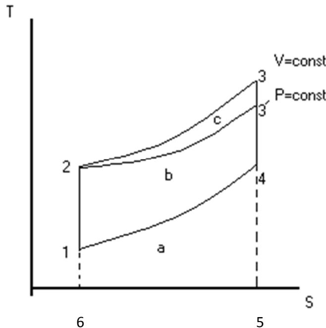
Heat input for Otto cycle  $Q_1$  is the area between the points (6,2,3,5,6),
