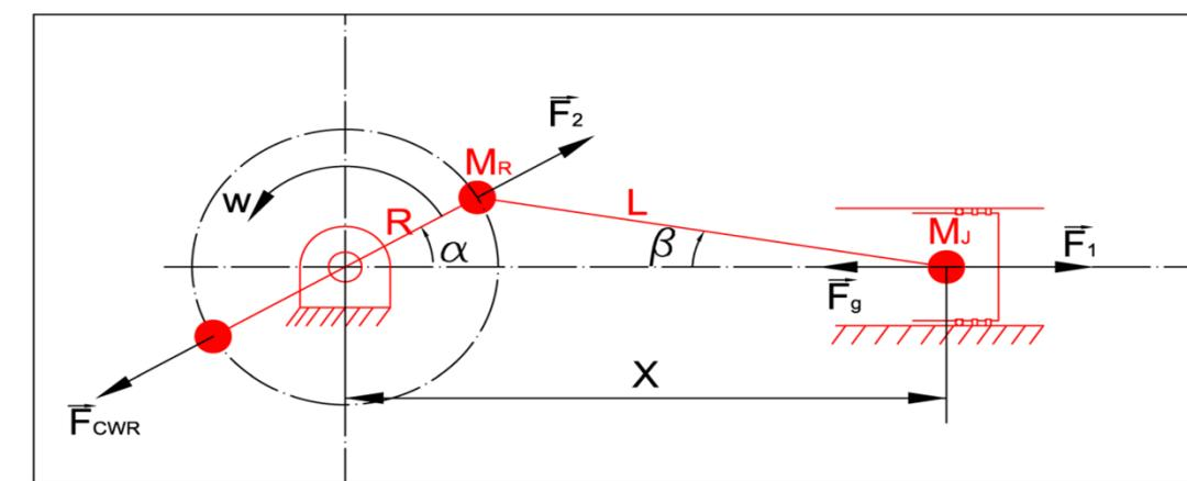
$$\overrightarrow{F_{cwR}} = |F_{cwR}| \angle \alpha + 180^\circ$$
