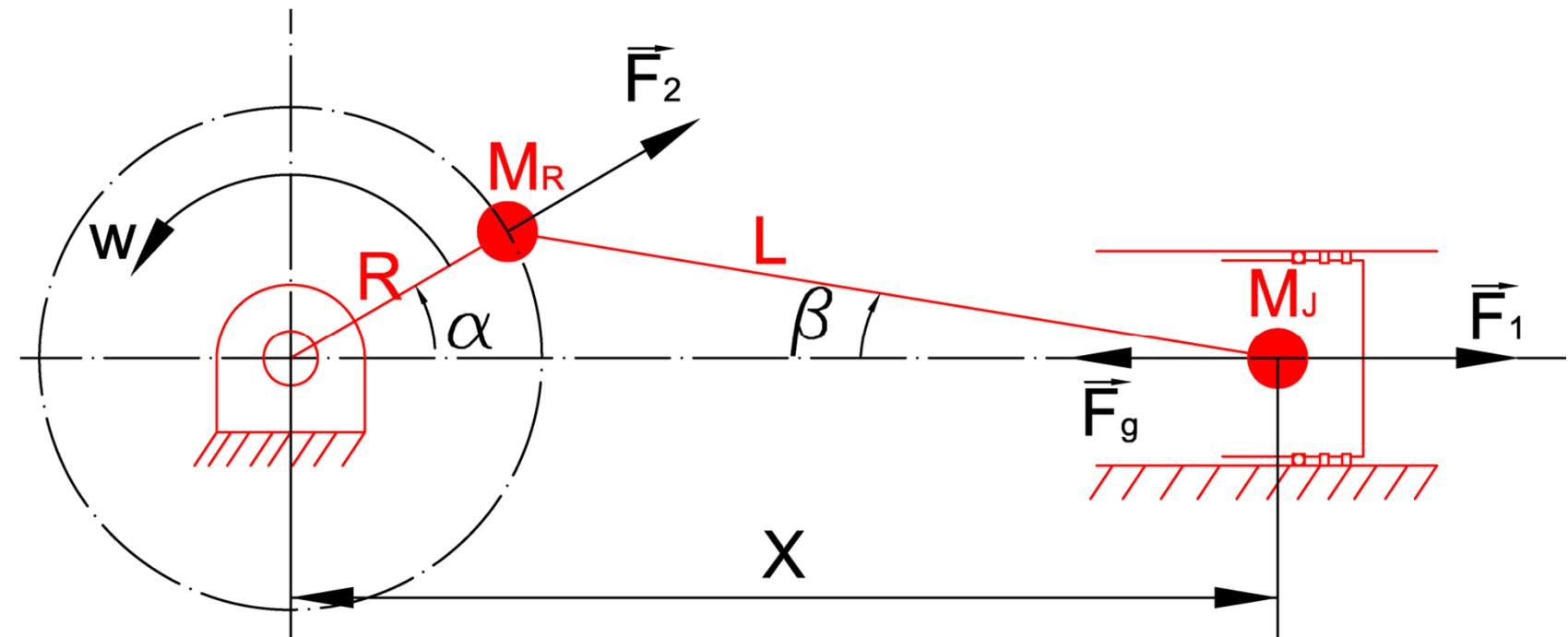
Total force acting on main bearings w/o balance
