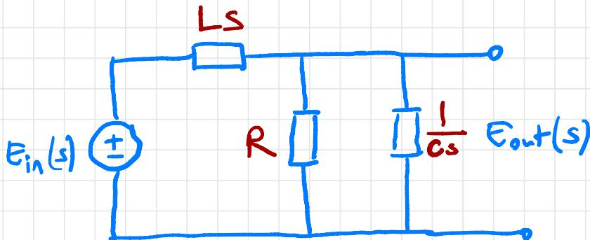
$$\frac{E_{out}(s)}{E_{in}(s)} = \frac{\frac{1}{cs} // R}{Ls + (R // \frac{1}{cs})} = \frac{\frac{1}{cs} \cdot R}{\frac{1}{cs} + R} \quad \text{Ls + } \left( \frac{\frac{1}{cs} \cdot R}{\frac{1}{cs} + R} \right)$$
