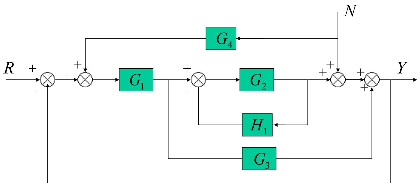
In this linear system, the output Y contains two parts, one part is related to R and the other is caused by N:
