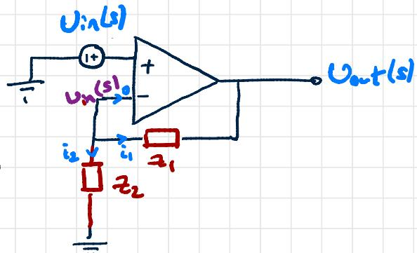
$$\begin{aligned} i_2 + i_1 &= 0 \\ \frac{U_{in}}{z_2} + \frac{U_{in} - U_{out}}{z_1} &= 0 \end{aligned}$$
