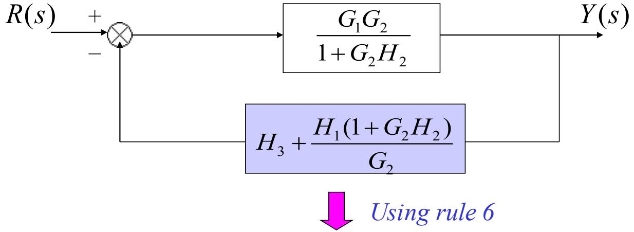
$$T(s) = \frac{Y(s)}{R(s)} = \frac{G_1 G_2}{1 + G_2 H_2 + G_1 G_2 H_3 + G_1 H_1 + G_1 G_2 H_1 H_2}$$
