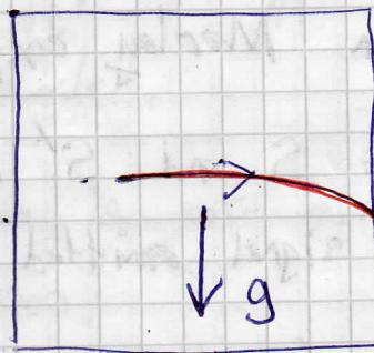
Equivalence principle requires that the path of a light should be curved in a frame at rest in a gravitational field with strength  $g$ .
