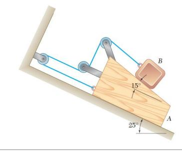
2) A 10-kg block B rests on a 5-kg bracket A, as shown below. The coefficients of friction are  $\mu_s = 0.40$  and  $\mu_k = 0.30$  between block B and bracket A, and there is no friction in the pulley or between the bracket and the horizontal surface. (a) Determine the maximum force F that can be applied if block B is not to slide on bracket A. (b) Determine the corresponding acceleration of the bracket A. (Answer :  $F_{max} = 24 N$ ,  $a_A = 1.6 m/s^2$ )
