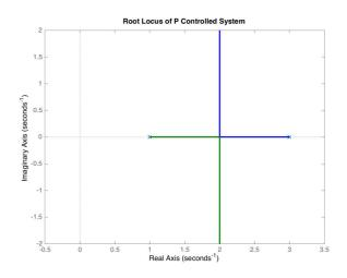
locus of the system with the following open-loop transfer function is plotted below after finding  $\sigma_a$  and  $\theta_a$  that are the intersecting point and angles with the real axis, respectively.
