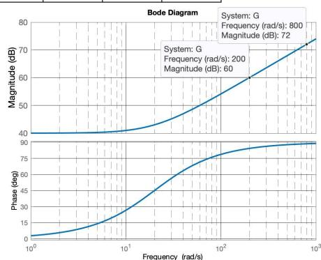
(e) We found that the linear gain at LF (dc gain) is  $K_{\text{lin}} = 40$  and break frequency is  $\omega_c = 20$  rad/s, which is the zero. Therefore, the transfer function that produces the above Bode plots should be,
