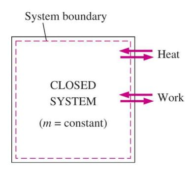
Energy can cross the boundaries of a closed system in the form of heat and work.
