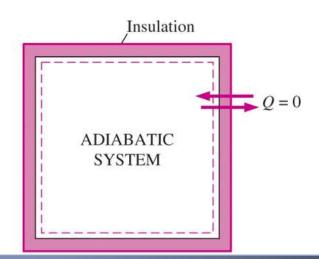
During an adiabatic process, a system exchanges no heat with its surroundings.
