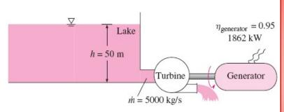
**Solution** A hydraulic turbine—generator is to generate electricity from the water of a lake. The overall efficiency, the turbine efficiency, and the shaft power are to be determined.
