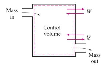
The energy content of a control volume can be changed by mass flow as well as heat and work interactions.
