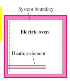
*Analysis* For this problem, the interior surfaces of the oven form the system boundary, as shown in Figure. The energy content of the oven obviously increases during this process, as evidenced by a rise in temperature. This energy transfer to the oven is not caused by a temperature difference between the oven and the surrounding air. Instead, it is caused by *electrons* crossing the system boundary and thus doing work. Therefore, this is a work interaction.
