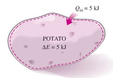
The increase in the energy of a potato in an oven is equal to the amount of heat transferred to it.
