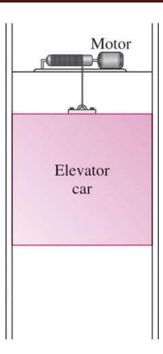
The energy transferred to a body while being raised is equal to the change in its potential energy.
