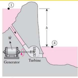
$$\dot{W}_{\text{max}} = \dot{m}\Delta e_{\text{mech}} = \dot{m}g(z_1 - z_4) = \dot{m}gh$$
