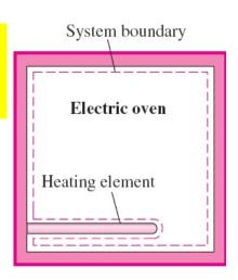
Analysis This time, the system boundary will include the outer surface of the heating element and will not cut through it, as shown in Figure. Therefore, no electrons will be crossing the system boundary at any point. Instead, the energy generated in the interior of the heating element will be transferred to the air around it as a result of the temperature difference between the heating element and the air in the oven. Therefore, this is a heat transfer process.
