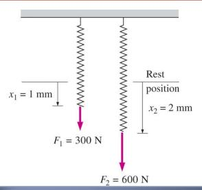
The displacement of a linear spring doubles when the force is doubled.
