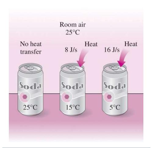
Temperature difference is the driving force for heat transfer. The larger the temperature difference, the higher is the rate of heat transfer.
