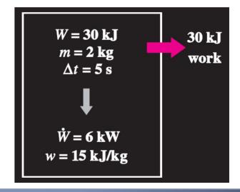
Power is the work done per unit time (kW)
