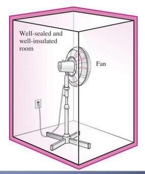
A fan running in a well-sealed and well-insulated room will raise the temperature of air in the room.
