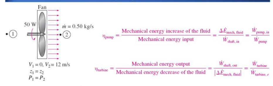
$$\eta_{\text{mech, fan}} = \frac{\Delta \dot{E}_{\text{mech, fluid}}}{\dot{W}_{\text{shaft, in}}} = \frac{\dot{m}V_2^2/2}{\dot{W}_{\text{shaft, in}}}$$
