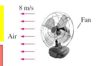
$$\dot{W}_{\rm elect, in} = \dot{m}_{\rm air} \, ke_{\rm out} = \dot{m}_{\rm air} \, \frac{V_{\rm out}^2}{2}$$
