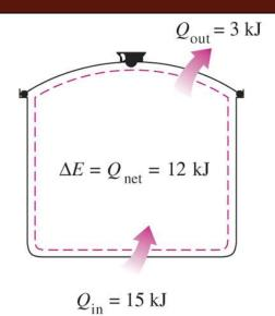
In the absence of any work interactions, the energy change of a system is equal to the net heat transfer.
