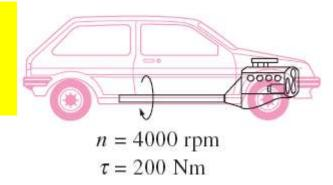
$$\dot{W}_{\rm sh} = 2\pi \dot{n} \text{T} = (2\pi) \left(4000 \frac{1}{\text{min}}\right) (200 \text{ N} \cdot \text{m}) \left(\frac{1 \text{ min}}{60 \text{ s}}\right) \left(\frac{1 \text{ kJ}}{1000 \text{ N} \cdot \text{m}}\right)$$
