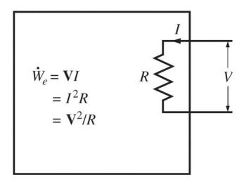
Electrical power in terms of resistance *R*, current *I*, and potential difference **V**.
