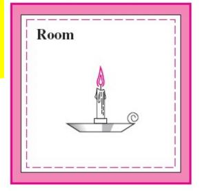
Analysis (a) The interior surfaces of the room form the system boundary, as indicated by the dashed lines in Figure. As pointed out earlier, heat is recognized as it crosses the boundaries. Since the room is well insulated, we have an adiabatic system and no heat will pass through the boundaries. Therefore, Q = 0 for this process.
