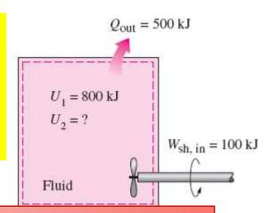
**Solution** A fluid in a rigid tank looses heat while being stirred. The final internal energy of the fluid is to be determined.
