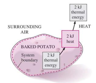
Energy is recognized as heat transfer only as it crosses the system boundary.
