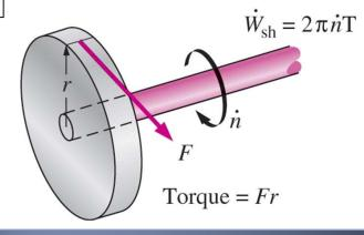
Shaft work is proportional to the torque applied and the number of revolutions of the shaft.
