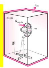
**Solution** A large fan is turned on and kept on in a room that loses heat to the outdoors. The indoor air temperature is to be determined when steady operation is reached. **Assumptions 1** Heat transfer through the floor is negligible.
