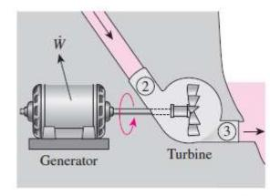
$$\dot{W}_{\text{max}} = \dot{m}\Delta e_{\text{mech}} = \dot{m}\frac{(P_2 - P_3)}{\rho} = \dot{m}\frac{\Delta P}{\rho}$$
