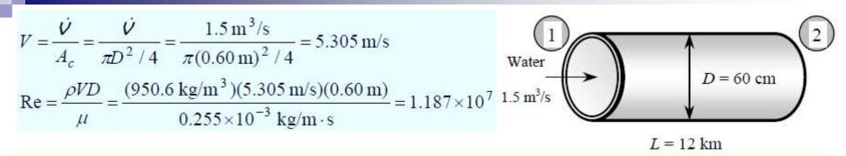
which is greater than 4000. Therefore, the flow is turbulent. The relative roughness of the pipe is
