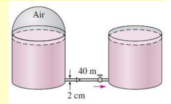
**Properties** The density and dynamic viscosity of water at 10°C are  $\rho$  = 999.7 kg/m³ and  $\mu$  =1.307×10<sup>-3</sup> kg/m·s. The loss coefficient is  $K_L$  = 0.5 for a sharp-edged entrance,  $K_L$  = 2 for swing check valve,  $K_L$  = 0.2 for the fully open gate valve, and  $K_L$  = 1 for the exit. The roughness of cast iron pipe is  $\varepsilon$  = 0.00026 m.
