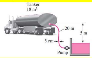
**Assumptions 1** The flow is steady and incompressible. **2** The entrance effects are negligible, and thus the flow is fully developed. **3** The flow is turbulent so that the tabulated value of the loss coefficients can be used (to be verified). **4** Fuel oil level remains constant. **5** Reservoir is open to the atmosphere.
