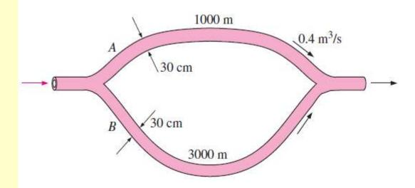
**Properties** The density and dynamic viscosity of water at 15°C are  $\rho$  = 999.1 kg/m³ and  $\mu$  =1.138×10<sup>-3</sup> kg/m·s. The roughness of cast iron pipe is  $\epsilon$  = 0.00026 m.
