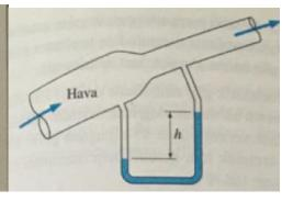
5-55 Air flows upward at a specified rate through an inclined pipe whose diameter is reduced through a reducer. The differential height between fluid levels of the two arms of a water manometer attached across the reducer is to be determined. √ Mod Feb'05.
