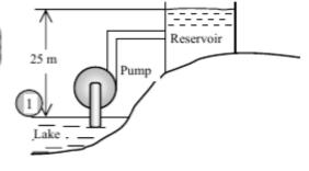
**Discussion** A more practical measure of performance of the pump is the overall efficiency, which can be obtained by multiplying the pump efficiency by the motor efficiency.
