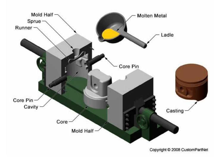
Permanent mould casting has the following limitations:
