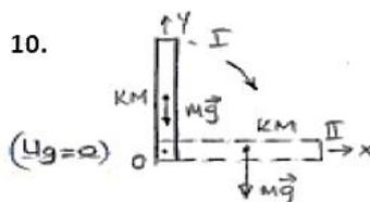
The moment of inertia of the rod through the center of mass:  $I_{KM} = \frac{1}{12} ML^2$
