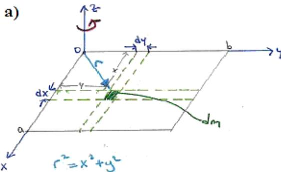
$$I_o = \int r^2 dm = \iint (x^2 + y^2) \sigma dx dy$$
