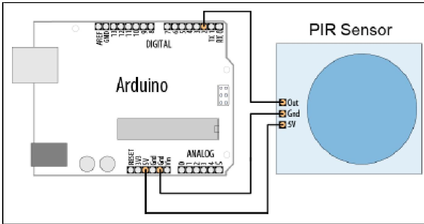
PIR sensors allow you to sense motion, almost always used to detect whether a human has moved in or out of the sensors range. They are often referred to as PIR, "Passive Infrared", "Pyroelectric", or "IR motion" sensors.
