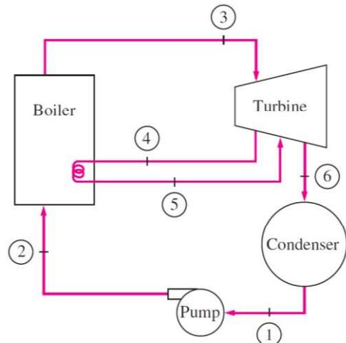
10-35 A steam power plant that operates on the ideal reheat Rankine cycle is considered. The pressure at which reheating takes place, the net power output, the thermal efficiency, and the minimum mass flow rate of the cooling water required are to be determined.
