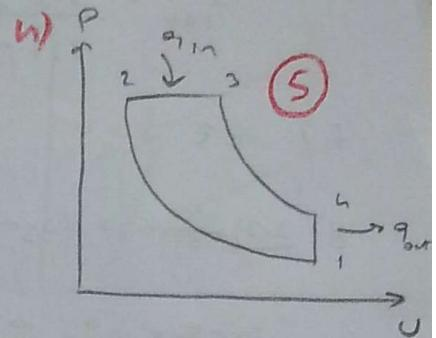
$$\frac{T_4}{T_3} = \left( \frac{U_3}{U_4} \right)^{\frac{1}{k-1}} \Rightarrow \frac{U_3}{U_4} = \frac{U_3}{U_2} \cdot \frac{U_2}{U_4} = 2.55 \cdot \frac{1}{16} \Rightarrow T_4 = 2000 \text{ K} \cdot \left( \frac{2.55}{16} \right)^{0.4} = 1076.4 \text{ K}$$
