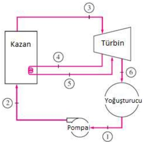
Steam enters the high-pressure turbine of a steam power plant that operates on the ideal reheat Rankine cycle at 6 MPa and 500°C and leaves as saturated vapor. Steam is then reheated to 450°C before it expands to a pressure of 7.5 kPa. Heat is transferred to the steam in the boiler at a rate of 60 MW. Steam is cooled in the condenser by the cooling water from a nearby river, which enters the condenser at 7°C.
