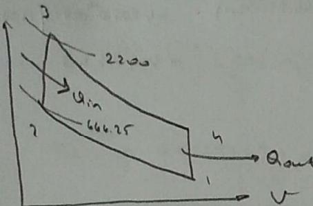
$$\frac{T_3}{T_4} = \left( \frac{V_4}{V_3} \right)^{\kappa-1}$$
