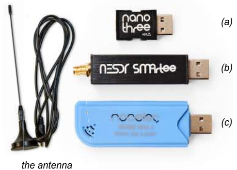
Figure 1.2: Three types of NooElec NESDR RTL-SDR: (a) the compact Nano 3 , (b) the RF shielded SMATee v2 , and (c) the Mini 2 ; and their antenna
