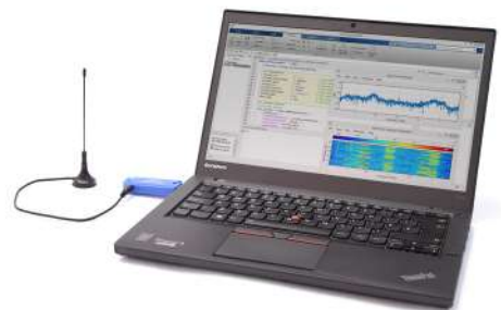
Figure 1.2: RTL-SDR with an omni-directional antenna connected to a laptop via a USB port. The computer is running MATLAB & Simulink to enable implementation of the DSP and SDR algorithms presented in this book. MathWorks tools can be used to monitor the signal in the frequency and time domains as it is demodulated [59]
