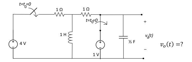
Obtain the  $v_o(t)$  voltage by using s-domain analysis.
