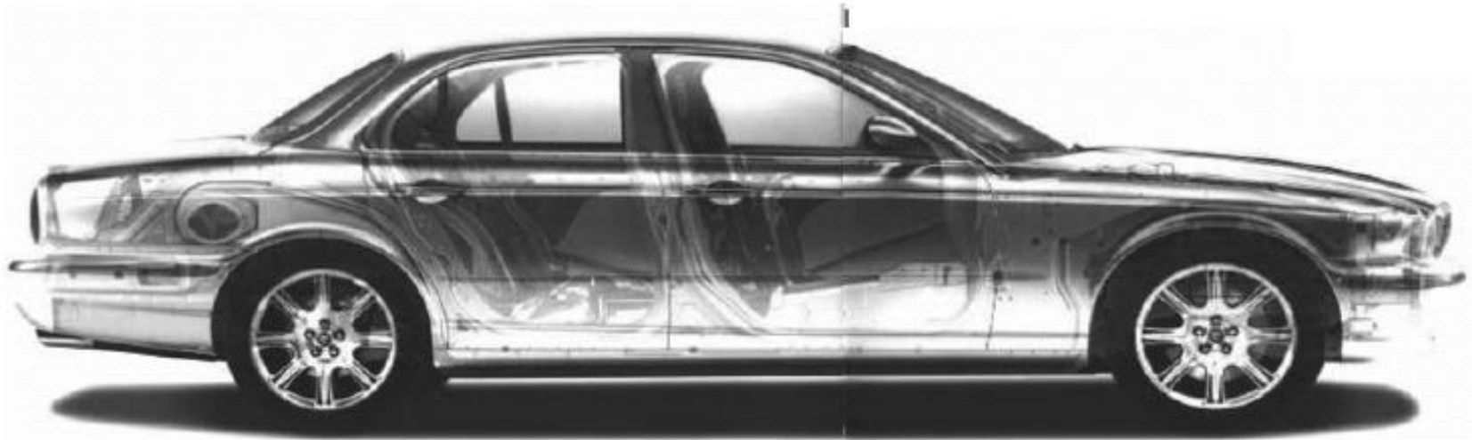
3.8 Schematic of the aluminum intensive Jaguar XJ2200 sport sedan with a monocoque body-in-white containing adhesively bonded and riveted stamped aluminum alloy sheet components. © Light Metal Age, reproduced with permission.
