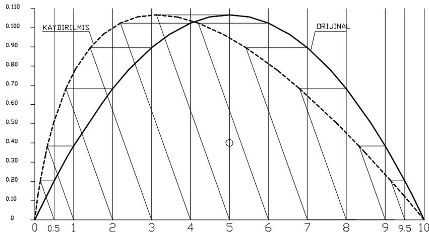
**Figure 6.16.** original and modified sectional area curves
