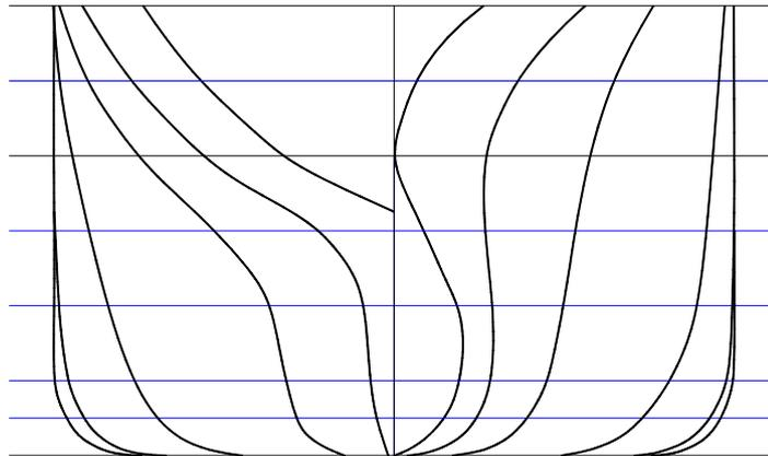
**Figure 6.32.** Body plan of the parent form
