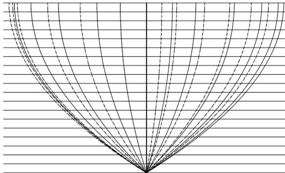
**Figure 6.17.** Body plan of the modified Wigley form
