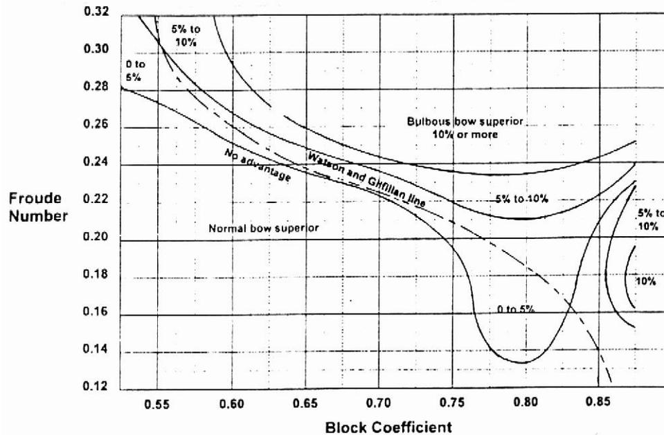
Figure 6.7. Criterion for bulbous bow according to Watson
