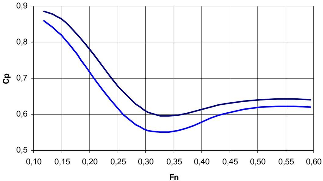
Figure 6.2. Prismatic coefficient as recommended by Saunders
