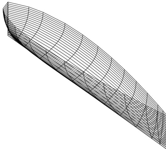
**Figure 6.18.** 3D view of the modified form
