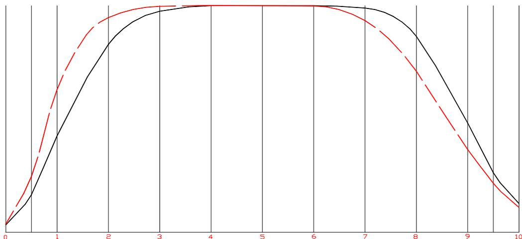
**Figure 6.20.** The basis and modified sectional area curves
