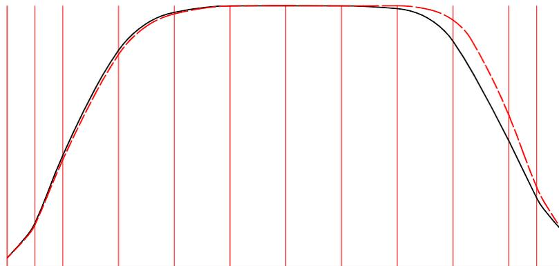
**Figure 6.33.** Original and modified sectional area curves
