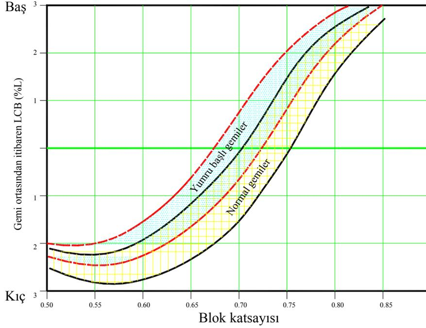
**Figure 6.6.** LCB position versus block coefficient
