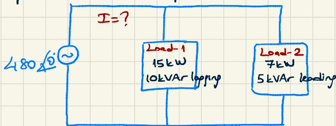
b)  $I = ?$        $S_1 \rightarrow \text{Inductive } (L) + \text{VAC}$        $S_2 \rightarrow \text{capacitive } (C) -$
