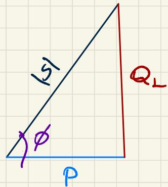
Ex: Two parallel loads draw from a 480 V (rms) source as shown below, where Load-1 draws 15 kW and 10 kVAr lagging, and Load-2 draws 7 kW and 5 kVAr leading. Determine the combined power factor and total apparent power drawn from the source.
