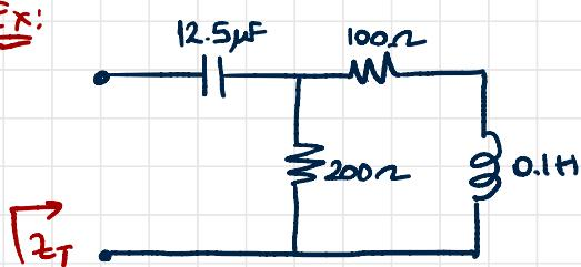
Determine the complex impedance between terminals shown in figure  $\omega = 1000 \frac{\text{rad}}{\text{s}}$
