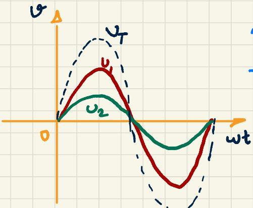
The addition (or subtraction) of two sinusoidal voltages of the same frequency and phase angle is simply the sum (or difference) of the peak values of each with the sum (or difference) having the same phase angle.
