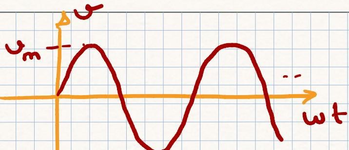
RMS of Sinusoidal Signal is  $\frac{V_m}{\sqrt{2}} = V_{rms}$
