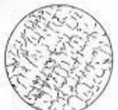
TYPE E Interdendritic flake graphite (hypo-eutectic compositions)
