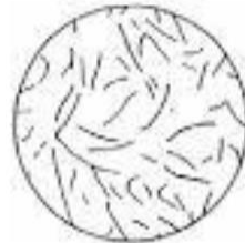
TYPE A Random flake graphite in a uniform distribution
