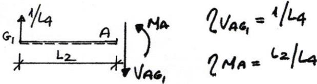
$$\begin{aligned} \sum V_{AG_1} &= 1/L_4 \\ \sum M_A &= L_2/L_4 \end{aligned}$$
