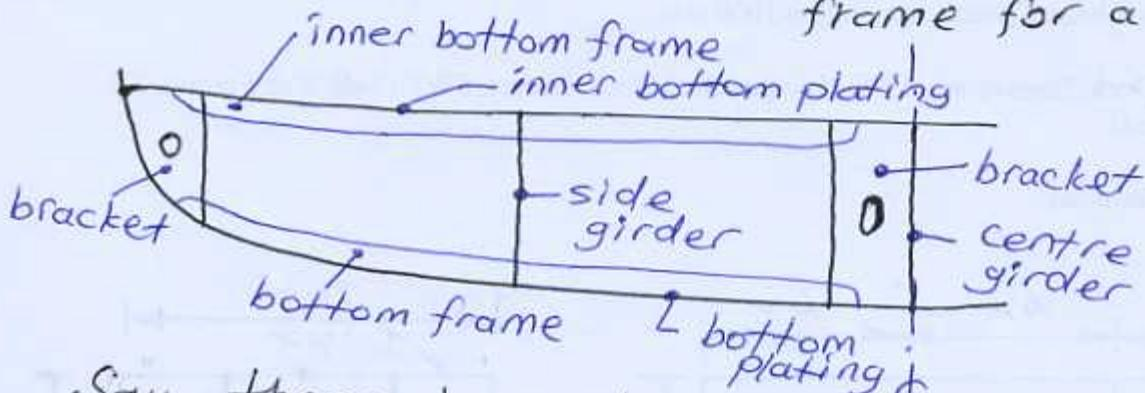
Say, there is only one side girder fitted each side. Then, unsupported span (length) will be approximately :
