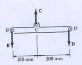
Solution. The factor of safety with respect to failure must be 3.0 or more in each of the three bolts and in the control rod. These four independent criteria will be considered separately.
