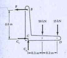
Free Body: Entire Bracket. The reaction at C is represented by its components  $C_*$  and  $C_w$ .
