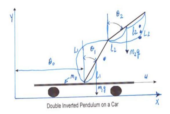
Subscripts 0,1,2 used with the aforementioned parameters refer to the cart, first (bottom) pendulum and second (top) pendulum correspondingly.
