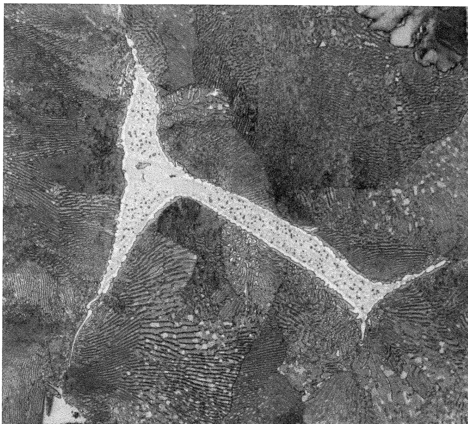
FIGURE 11.6 Optical micrograph of steadite (iron-iron phosphide eutectic in gray cast pig iron). (From Vander Voort [3].)
