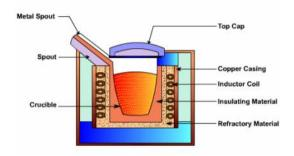
Figure 16: Schematic of a Induction Furnace
