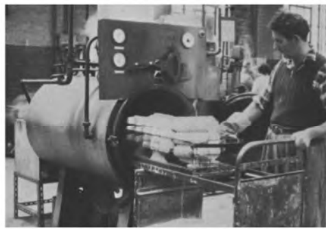
Dewaxing the ceramic shell moulds in a steam autoclave. (Courtesy of BSA Precision Castings Ltd.)
