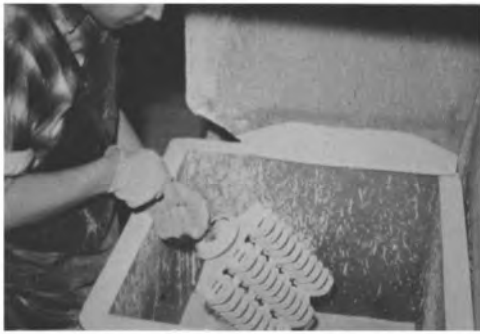
Application of the stucco in a fluidised bed of refractory (ceramic shell process). (Courtesy of BSA Precision Castings Ltd.)
