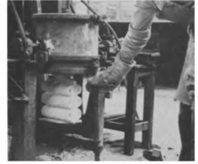
Casting the fired ceramic shell mould (the indirect arc furnace has been rotated through 180° to cast the mould, ie the Durville method of casting). (Courtesy of BSA Precision Castings Ltd.)
