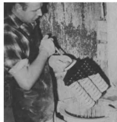
Application of the primary dip-coat slurry by dipping the pattern assembly. (Courtesy of BSA Precision Castings Ltd.)
