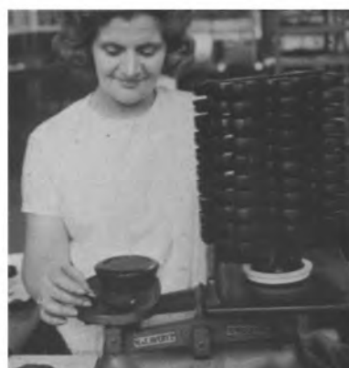
Completed wax pattern assembly. The operative is checking the weight of the assembly which comprises 60 individual patterns. (Courtesy of BSA Precision Castings Ltd.)
