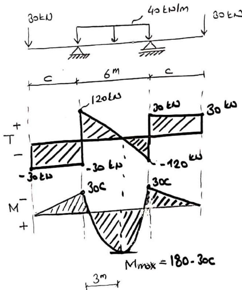
$M_{max} = 180 \cdot 30c$  [kNm] at middle of the beam span
