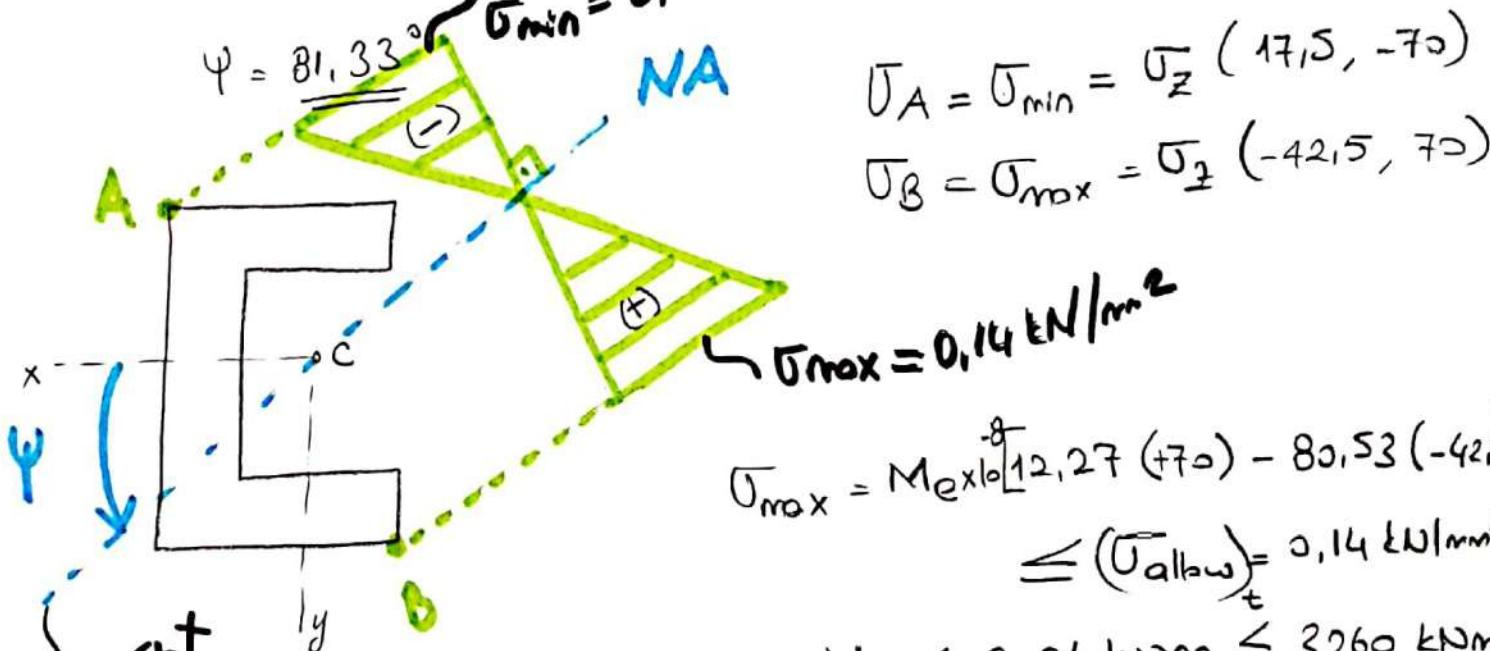
$$\bar{\sigma}_A = \bar{\sigma}_{min} = \sigma_z (17.5, -70)$$
