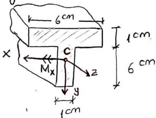
The cross-sectional area is symmetric about "y" axis that is perpendicular to the neutral axis on which the moment "M" acts alone.
