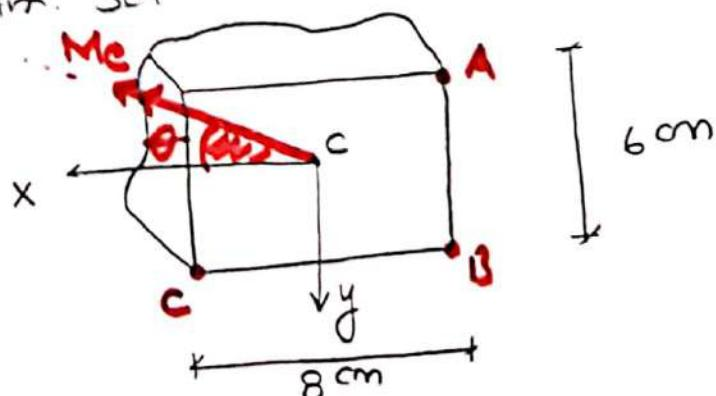
(a) Due to symmetry with respect to x and y axes, no need to determine the centroid of the cross-section. Moments of inertia of the cross-sectional area about the x and y axis must be determined, respectively.
