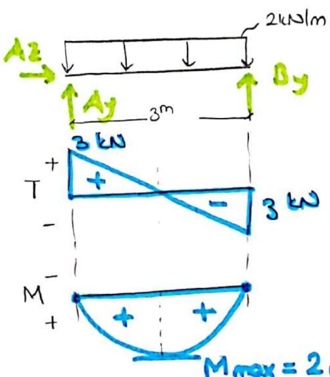
$$M_{max} = 2.25 \text{ kNm} \quad (\text{at the middle point of the beam span})$$
