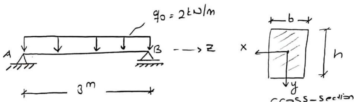
There is symmetry with respect to x and y axis. So no need to calculate the centroid for the member's cross-sectional area. The neutral axis is also the horizontal centroidal axis for the cross-section.
