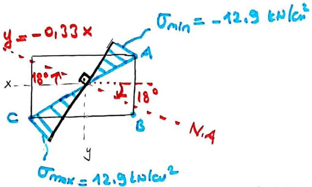
Normal stress distribution will be drawn along a line that is perpendicular to NA.
