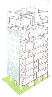
relatively straightforward: The existing thickness of the wood panels, combined with a layer of drywall, allowed the design team to achieve fire resistance ratings of 60 and 90 minutes.
