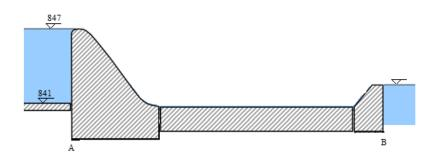
**7.17.** A diversion weir as seen in Figure is planning to construct on a fine-gravel bed. Make analyzes of the diversion weir with using the Lane method (C = 4). Determine the length of the sheet pile. Control the width of the stilling basin if it is sufficient or not.
