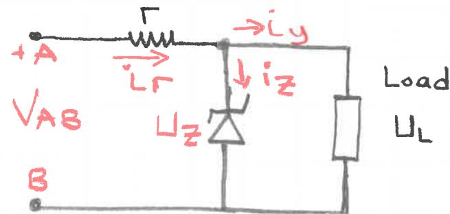
$$I_{Z\min} = \frac{V_{AB\min} - U_Z}{r} - I_{y\max}$$
