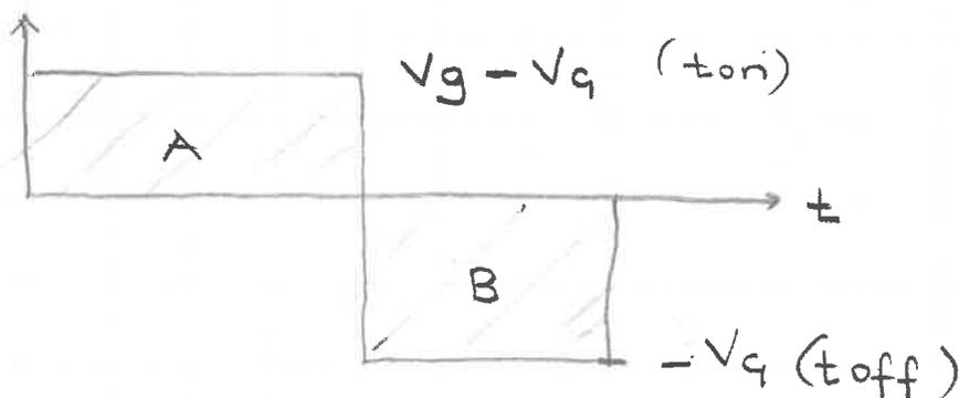
The calculation based on voltage  $\times$  time balance
