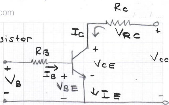
a) By taking  $R_B = 80 \Omega$  and  $V_{BE} = 1 \text{ V}$ , calculate base current ( $I_B$ ), collector current ( $I_C$ ), Load voltage ( $V_{RC}$ ) and transistor voltage ( $V_{CE}$ ).
