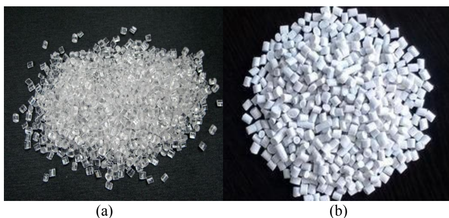
Figure 5: (a) General purpose crystal PS and (b) anti-shock PS.
