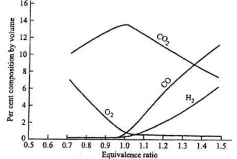
Even if the unburned fuel and oxygen combine later during the expansion stroke, resulting in no loss of fuel in the exhaust, still there will be a loss in efficiency, since the sensible energy present with the combustion of this part of fuel is not utilized at top dead center and hence does not contribute to the pressure rise at that point.
